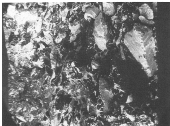
Figure 3 Fracture surface of composite containing 25% SBR50. \times 27 .
