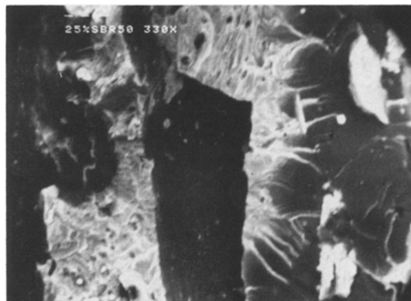
Figure 4 Fracture surface of composite containing 25% SBR50. \times 220 .
